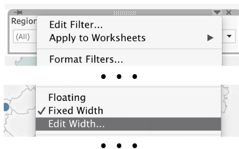
Figure 2. Menu for editing the width of a filter widget
