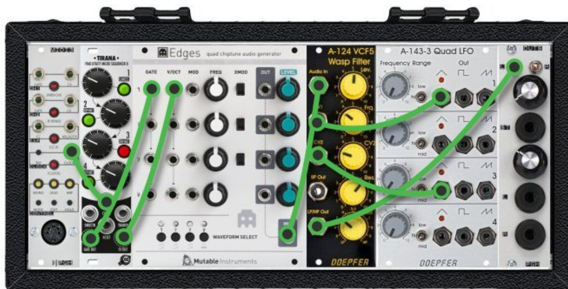
Figure 2 Example modular patch. Screenshot of modularGrid.com. From left to right the modules are MIDI (as clock source); micro-sequencer; Edges oscillator bank; Wasp filter; Quadruple LFO; Outputs.
