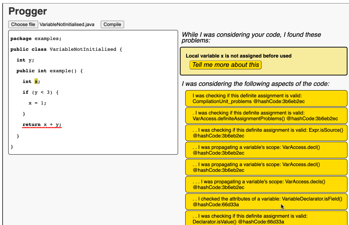
Figure 4. Screenshot of the Progger prototype showing an expanded error view. The highlighted variable ( x ) corresponds to the code location investigated while evaluating the attribute where the cursor is hovering.
