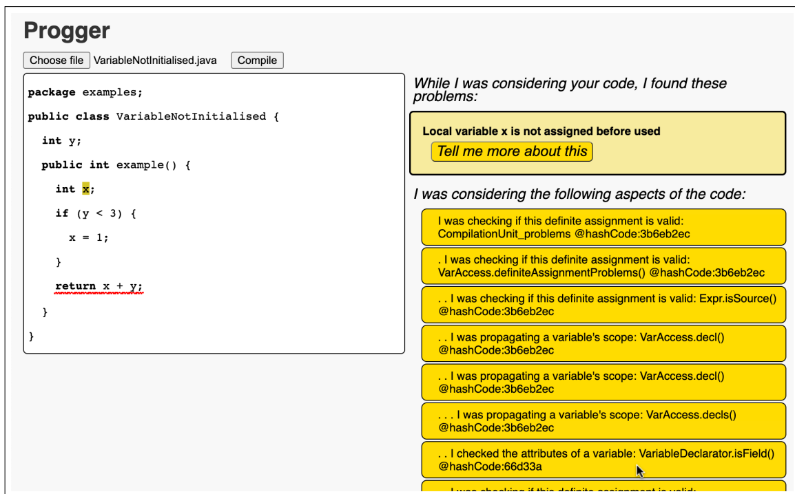
Figure 2 – Screenshot of Progger version 1.0. The left side shows a small Java code snippet with an error in it pointed out with a red squiggly line. The right side shows the error with a "Tell me more about this" button which has been clicked here to expand an attribute trace tree shown in the bottom right.
