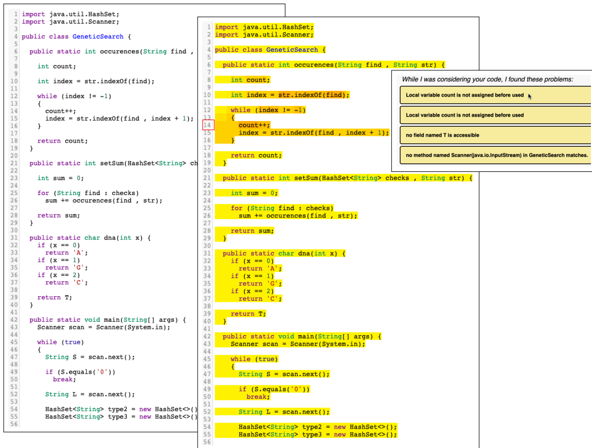
Figure 8 – An example of a heat map generated on a one of the Java code snippet that was presented in the user study. As the mouse pointer is hovering over the first error ("local variable count is not assigned before use" on line 14) the attention of the compiler when finding that error is shown is visualized as a line-based heat map.
