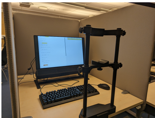
Figure 2 – The experimental setup. The apparatus is contained within a booth, with the eye-tracker visible below the screen and a chin- and forehead rest in the foreground.
